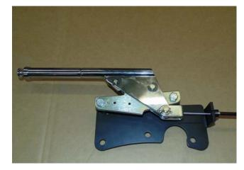
4. Slide cable housing over cable and locate front housing end in housing locator on the handle bracket.
