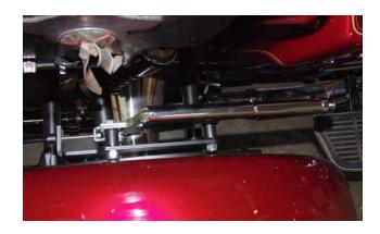
6. Mark the length of the housing. Cable needs to be longer than the housing. Do not cut the cable now. Remove housing from the cable. Use an abrasive cut off wheel to cut the housing. Do not Smash the housing
