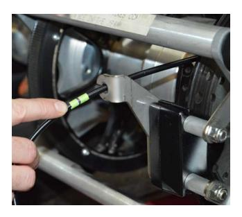
7. Install cable clevis on caliper actuator lever.
